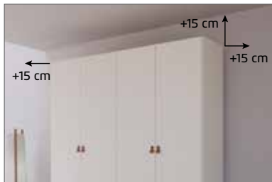
The following space is required to mount the wardrobe: wardrobe height + min. 15 cm, wardrobe width + min. 15 cm on each side.
